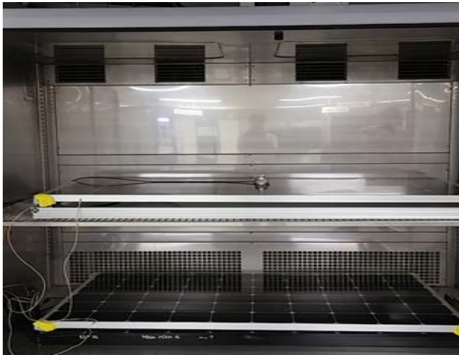
Figure 5: PID Test with Light source
